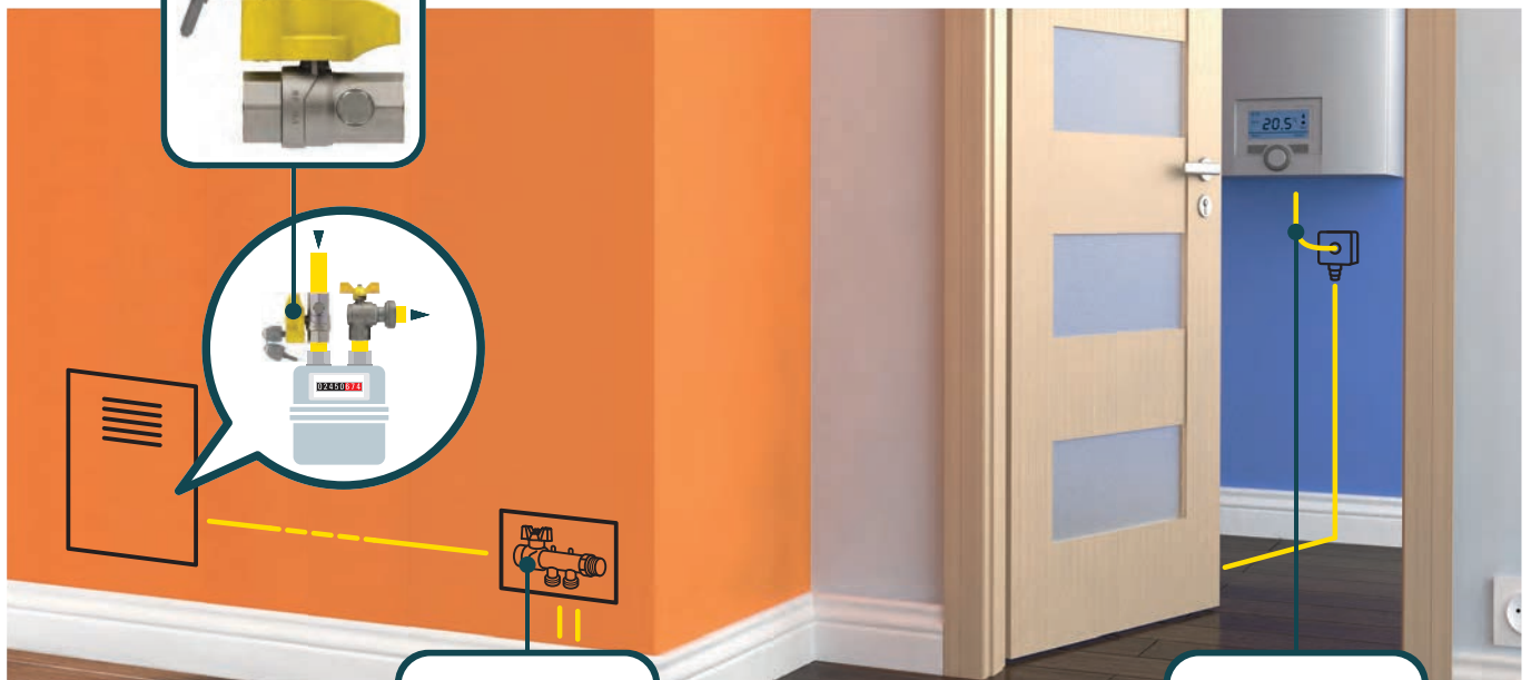
Covered flexible pipes in AISI stainless steel
